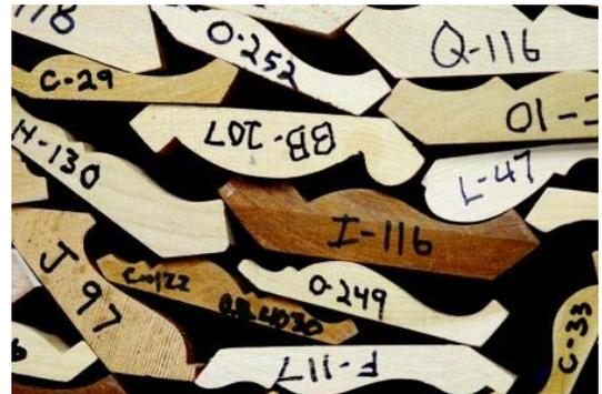
**Set up Costs** are determined by the complexity of the profiled part to be manufactured, In addition to installing cutter heads on the machine, fences, chip breakers and pressure hold down shoes must be set and adjusted. On longer runs and for abrasive materials such as Teak, frequent re-sharpening of knives is also required.
